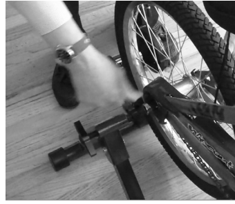
Tighten inside wing nuts (13)
