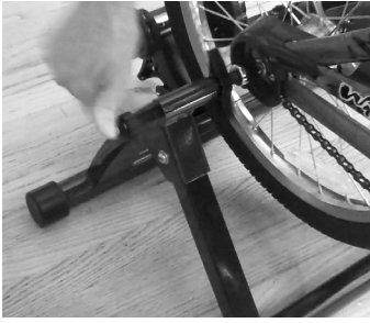
Tighten outside wing nuts (12)
