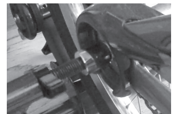
Position hub clamps (11) on wheel axle bolts (both sides)
