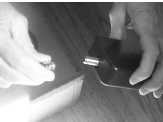
Attach it to one end of the 123GoTV receiver (3). Attach the 123GoTV coaxial cable (4) to the other end of the receiver.
