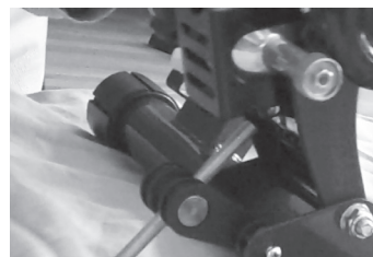
Turning clockwise insert and tighten resistance knob into the hole
