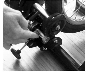
Good contact is when generator (2) moves with wheel. Don't overtighten.
